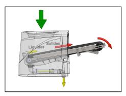
Toilet Tech Solutions offers a completely enclosed, single unit, mechanical foot-operated, urine-diverting toilet system. This unit can be installed in less than 20 minutes into a simple site built toilet structure, solids treatment zone (behind the wall), and urine pipe. Urine can go to a simple septic field, sewer drain, storage tank for sanitization and reuse, or to a constructed wetland.
